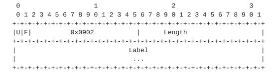
See [GMPLS-SIG] for a description of parameters and encoding of SDH, SONET, port, wavelength and other labels.
