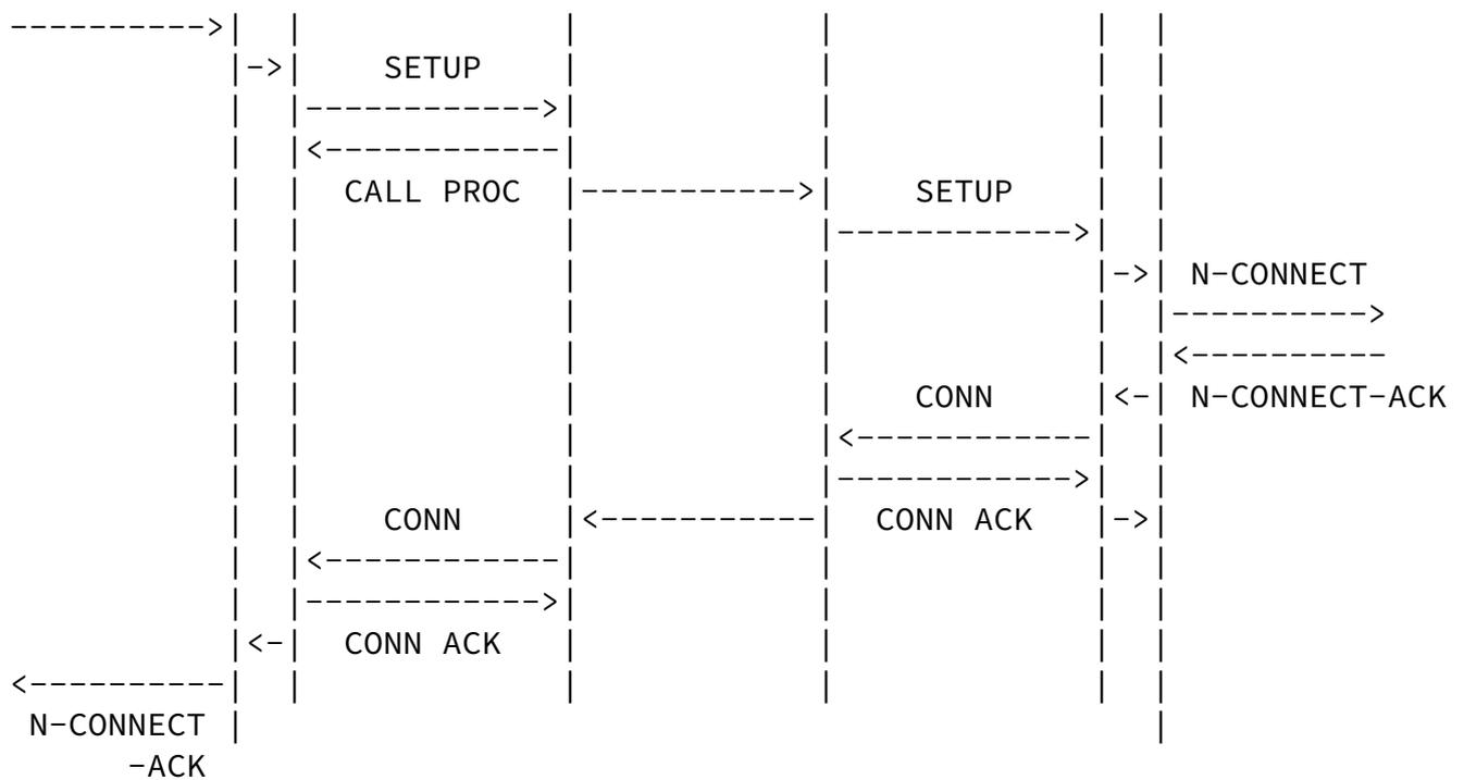
Fig. 2.2: Example procedure for simultaneous QoS-sensitive session and ATM VC establishment.
