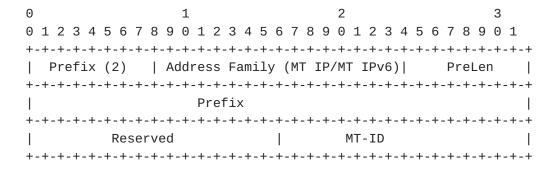
Figure 2: MT Prefix FEC Element Format
