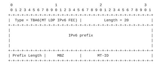
Figure 7: MT LDP IPv6 FEC sub-TLV
