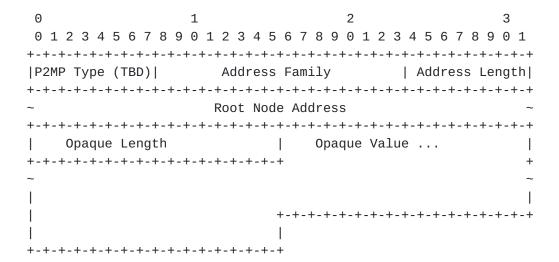
Type: The type of the P2MP FEC Element is to be assigned by IANA.
