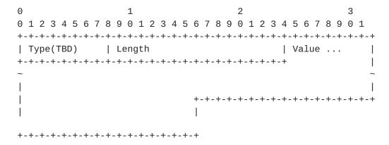
Type: The type of the LDP MP Opaque Value Element is to be assigned by IANA.
