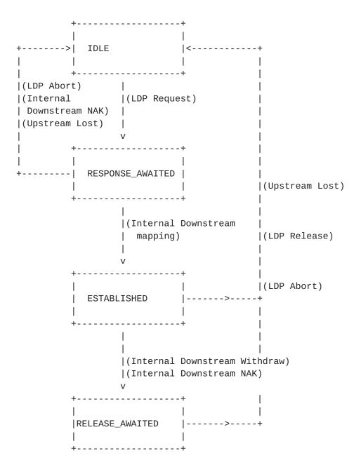
3.2.3.4 Upstream\_LSP\_Control\_Block's State Machine for Downstream-on-demand Mode
