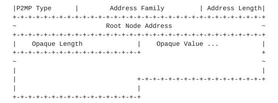
The Address Family MUST be set to IPv4, the Address Length MUST be set to 4 and the Root Node Address MUST be set to an IPv4 address when the LDP P2MP LSP TLV is carried in the IPv4 Interface ID TLV. The Address Family MUST be set to IPv6, the Address Length MUST be set to 16 and the Root Node Address MUST be set to an IPv6 address when the LDP P2MP LSP TLV is carried in the IPv6 Interface ID TLV.
