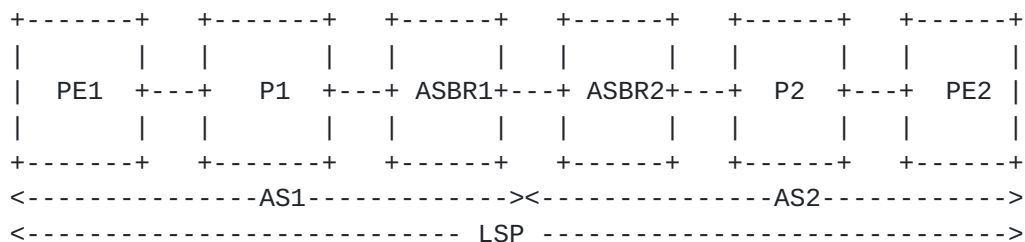
Figure 1: Simple Inter-AS LSP Configuration
