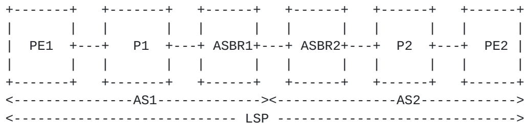
Figure 1: Simple Inter-AS LSP Configuration
