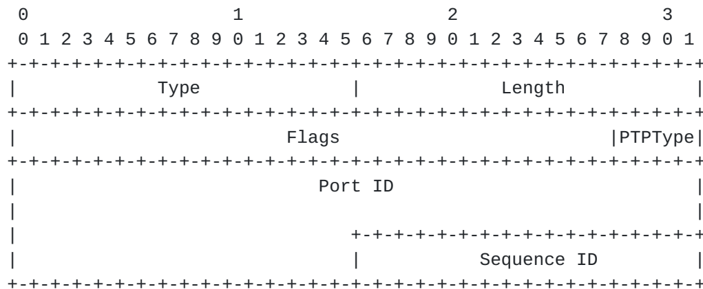
Figure 2: PTP Sub-TLV format
