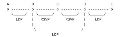
When an LSP traceroute is initiated from Router A to Router E, the FEC information included in the packet will be LDP while Router C along the path is a pure RSVP node and does not run LDP. Consequently, node C will be unable to perform FEC validation. The MPLS echo request should contain sufficient information to allow any transit node within stitched or tunneled LSP to perform FEC validations to detect any misrouted echo request.
