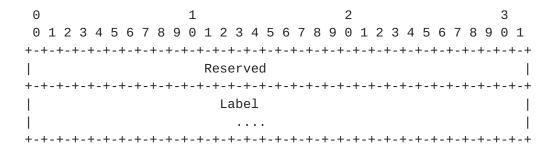
The label can be encoded as in [RFC3209] when the C-Type is 1 or as a Generalized Label [RFC3473] when the C-Type is 2 or 3.
