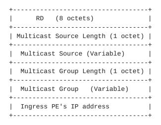
RD is set to 0 for (S,G) state and all 1s for (\*,G) state, Multicast Source is set to S for (S,G) state or RP for (\*,G) state, Multicast Group is set to G, Multicast Source Length and Multicast Group Length is set to either 4 or 16 (depending on whether S/RP and G are IPv4 or IPv6 addresses).
