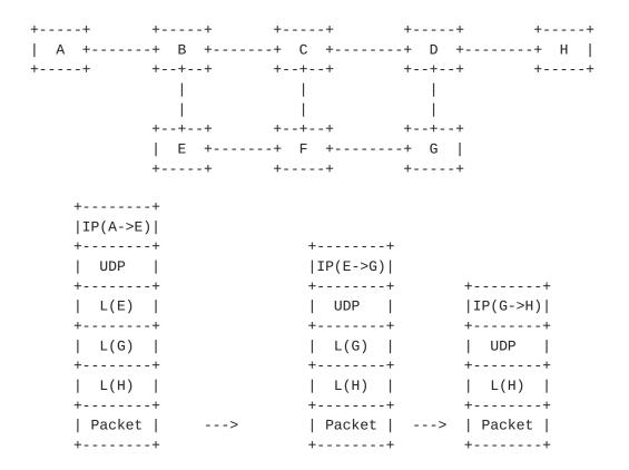
Figure 4: Packet Forwarding Example without PHP
