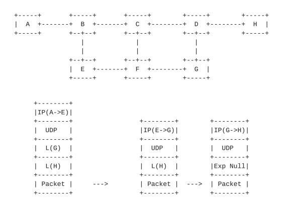
Figure 3: Packet Forwarding Example with PHP
