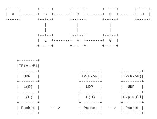
Figure 3: Packet Forwarding Example with PHP
