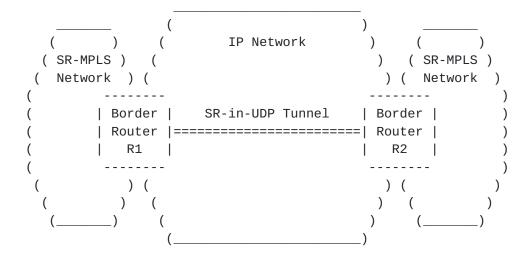
Figure 1: SR-MPLS in UDP to Tunnel Between SR-MPLS Sites
