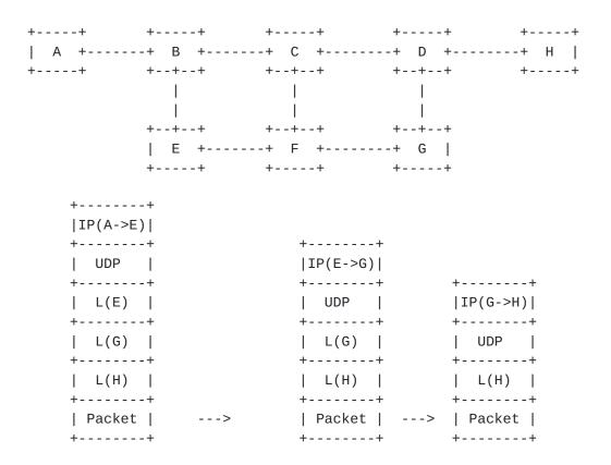
Figure 4: Packet Forwarding Example without PHP
