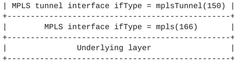
In the above diagram, "Underlying Layer" refers to the ifIndex of any interface type for which MPLS internetworking has been defined. Examples include ATM, Frame Relay, and Ethernet.
