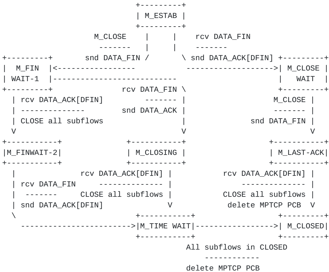
Figure 17: Finite State Machine for Connection Closure
