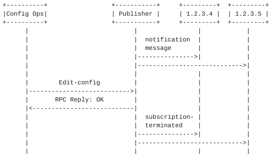
Figure 16: Interaction model for configured subscription deletion
