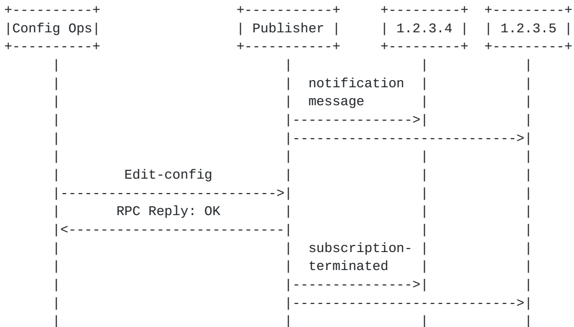
Figure 16: Interaction model for configured subscription deletion
