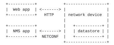
The following figure shows the system components if a RESTCONF server is implemented in a device that does not have a NETCONF server:
