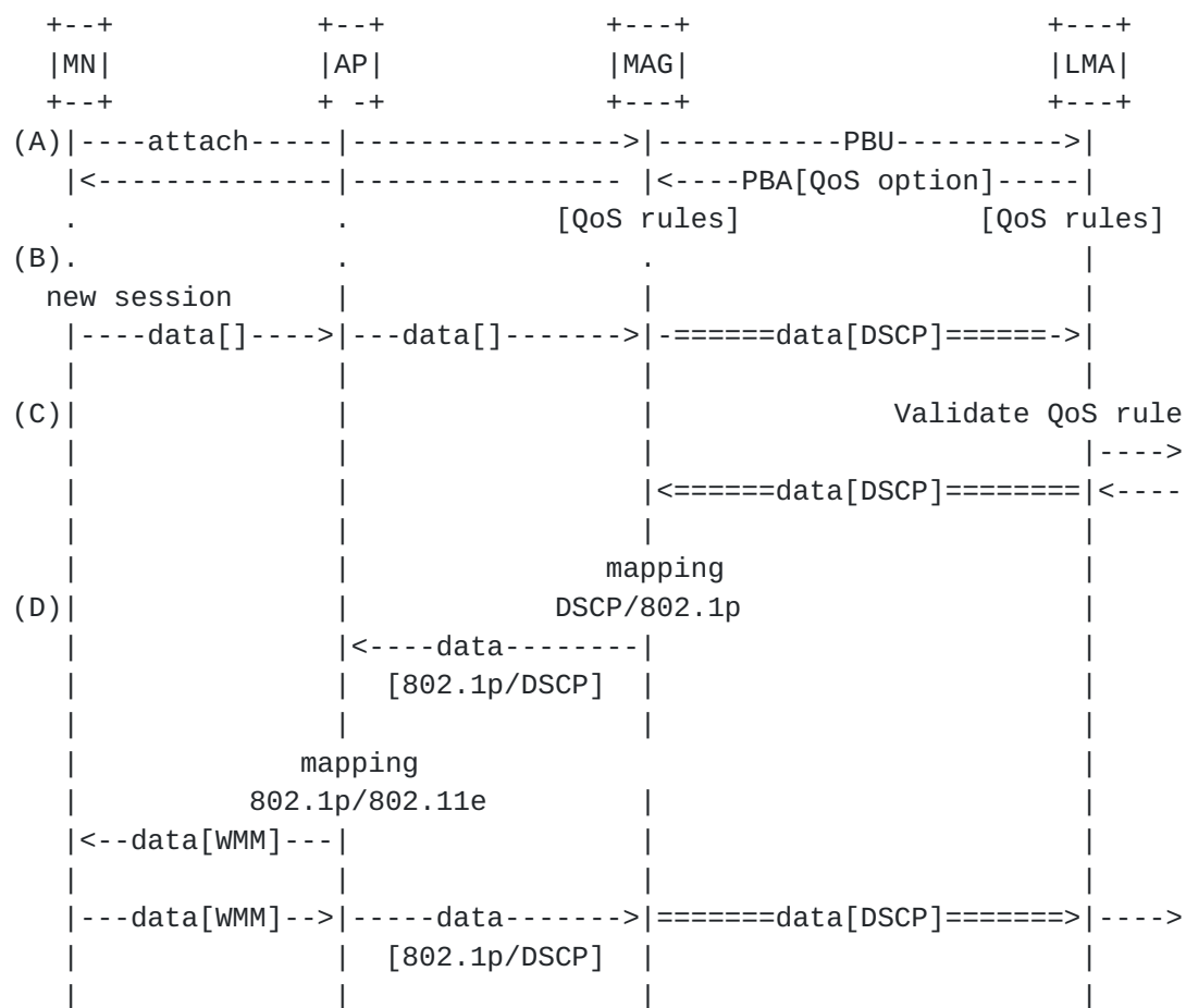
Figure 8: Prioritization of a flow created on the WLAN access
