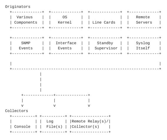
Figure 1. Syslog Processing Flow
