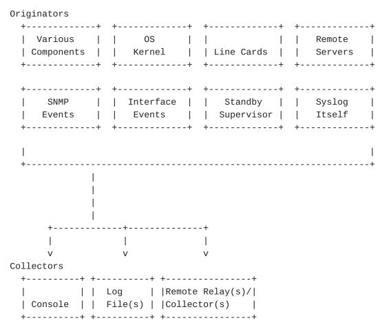
Figure 1. Syslog Processing Flow
