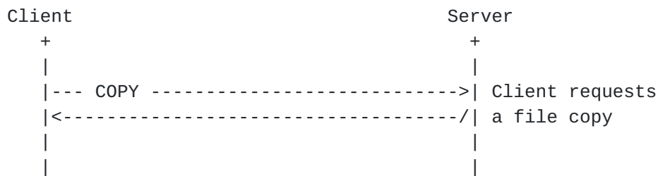
Figure 1: A synchronous intra-server copy.
