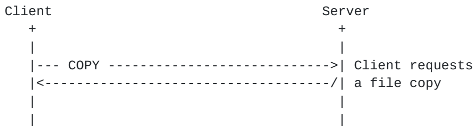
Figure 1: A synchronous intra-server copy.
