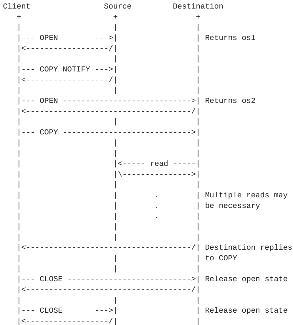
Figure 4: A synchronous inter-server copy.
