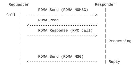
An RPC-over-RDMA transaction using a Long Reply:
