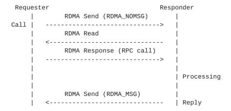
An RPC-over-RDMA transaction using a Long Reply:
