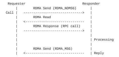
An RPC-over-RDMA transaction using a Long Reply:
