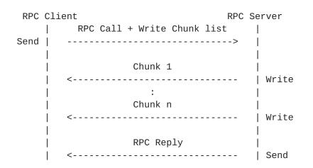
In the presence of write chunks, RDMA ordering provides the guarantee that all data in the RDMA Write operations has been placed in memory prior to the client's RPC reply processing.
