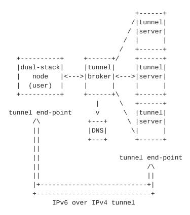
Figure 1: the Tunnel Broker model
