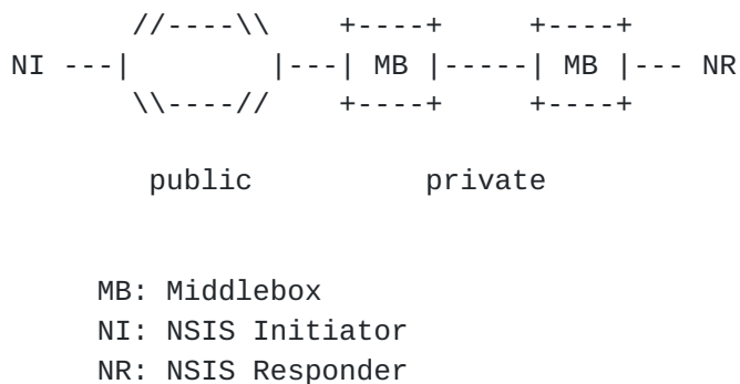
Figure 5: NAT with Private Network on Receiver Scenario
