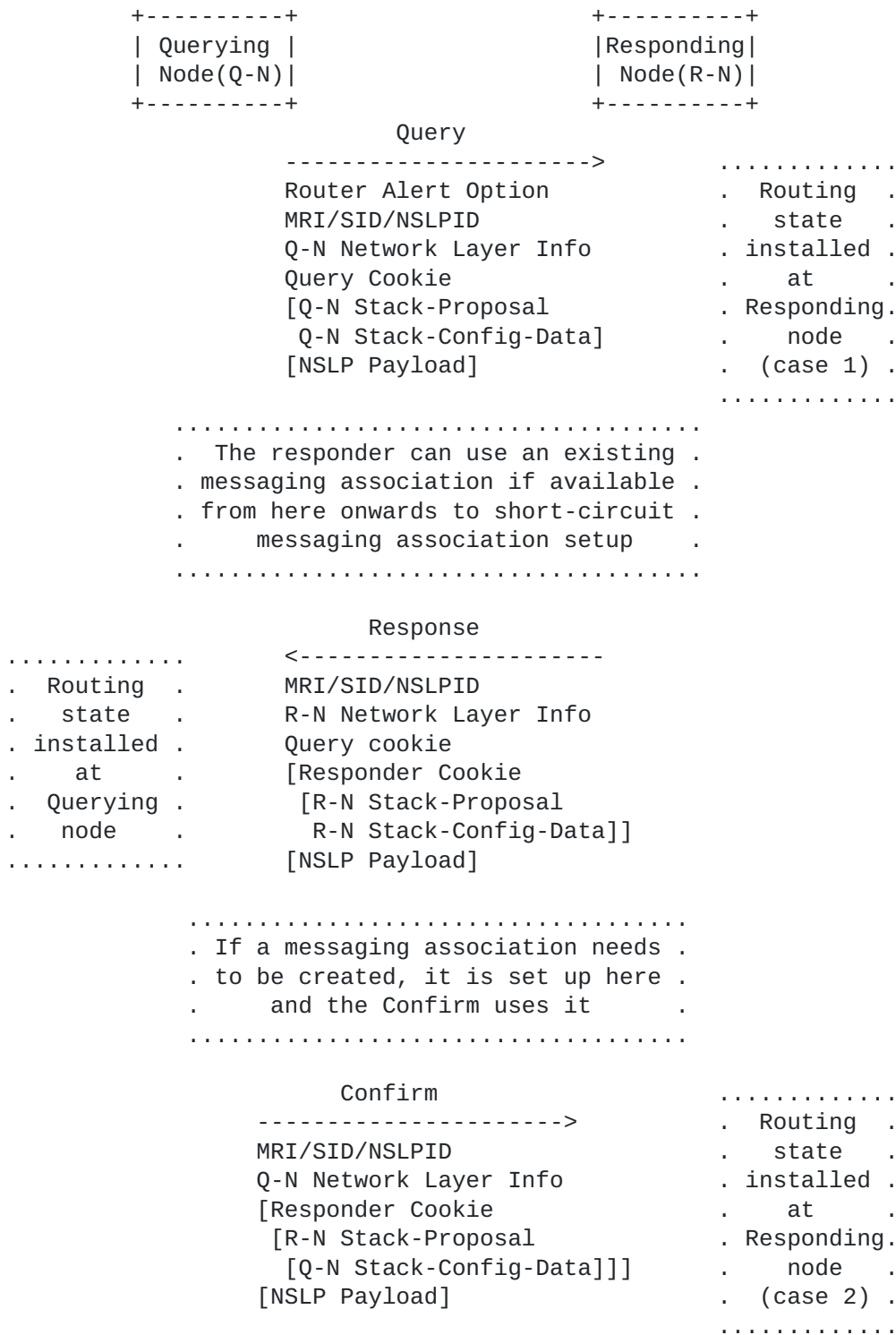
Figure 4: Message Sequence at State Setup
