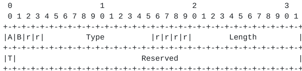
Figure 10: NODE_CAPABILITY Object Format
