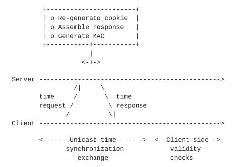
Procedure for unicast time synchronization exchange.
