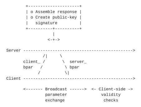
Procedure for unicast time synchronization exchange.
