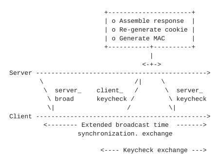
Procedure for extended broadcast time synchronization exchange.
