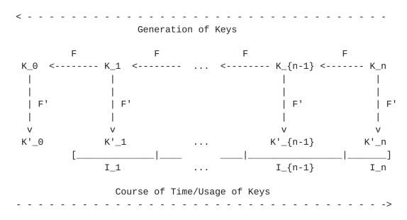
A schematic explanation of the TESLA protocol's one-way key chain
