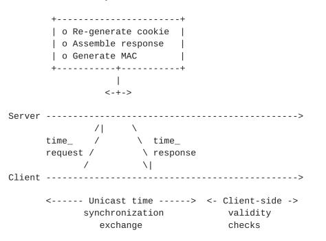
Procedure for unicast time synchronization exchange.
