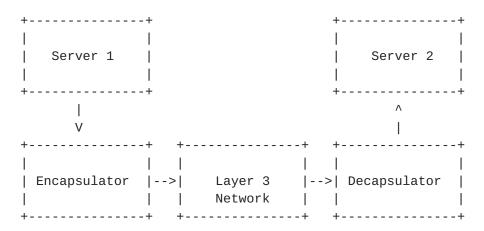
The encapsulator and decapsulator may be co-resident with the corresponding servers, or may be on separate nodes in the network.
