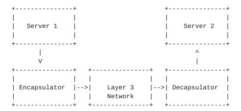
The encapsulator and decapsulator may be co-resident with the corresponding servers, or may be on separate nodes in the network.
