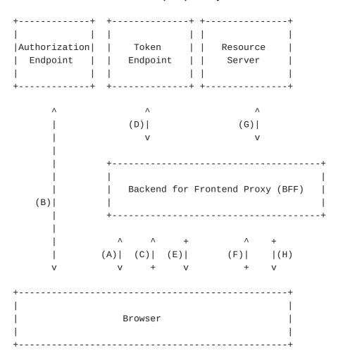
In this architecture, commonly referred to as "backend for frontend" or "BFF", the JavaScript code is loaded from a dynamic Application Server (A) that has the ability to execute code and handle the full authentication flow itself. This enables the ability to keep the call to actually get an access token outside the JavaScript application.
