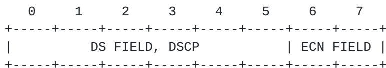
Figure 6: The Differentiated Services and ECN fields in IP
