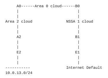
where A0 and B0 are area 0 border routers attached to Area 2 and NSSA 1 respectively. A2 and B1 are ASBRs. A2 advertises a route to 10.0.13.0 through E2 while B1 advertises a preferred Type 7 NSSA internal default through E1. Since NSSAs do not import Type 5 LSAs, NSSA 1 has no knowledge of the path through Area 2 to 10.0.13.0/24 and would instead choose to forward traffic destined to 10.0.13.0/24 to its Internet default through E1.
