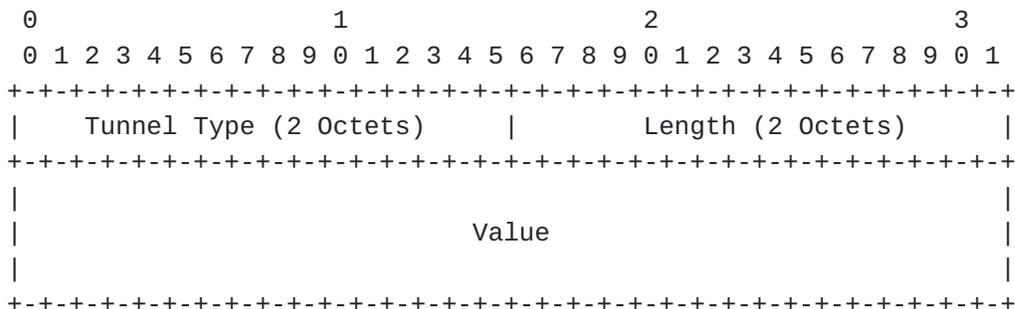
Tunnel Type (2 octets): identifies the type of tunneling technology being signaled. This document defines the following types:
