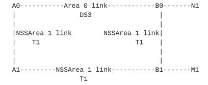
where A0 and B0 are border routers attached to NSSArea 1. A1 and B1 are internal routers in NSSArea 1. N1 and M1 are standard ethernet networks in NSSArea 1 directly attached to B0 and B1 respectively. Assume all T1 links have an OSPF cost of 28 in both directions, N1 and M1 are attached with interface costs 2. The DS3 link has an OSPF cost of 1. All costs are symmetric. Under the current OSPF specification the preferred path between A0 and M1 is
