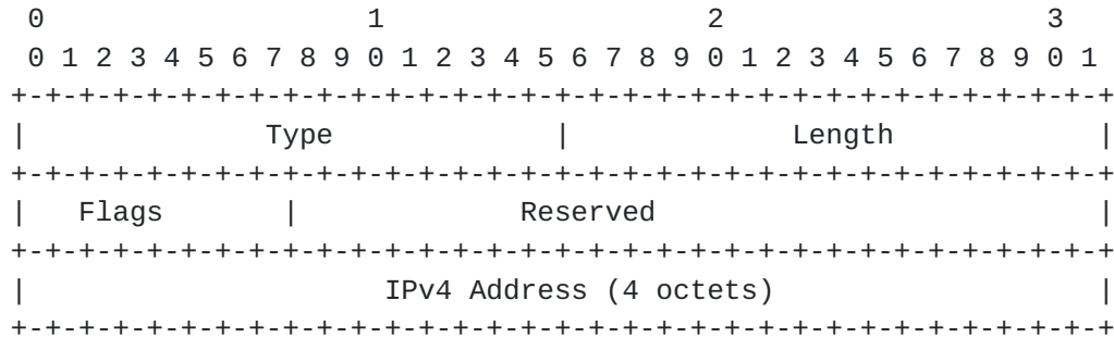
IPv4 Backup ERO sub-TLV format
