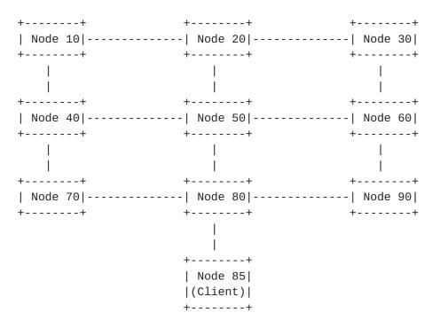
Because the graph is not fully connected, when a node wants to send a message to another node, it may need to route it through the network. For instance, Node 10 can talk directly to nodes 20 and 40, but not to Node 70. In order to send a message to Node 70, it would first send it to Node 40 with instructions to pass it along to Node 70. Different overlay algorithms will have different connectivity graphs, but the general idea behind all of them is to allow any node in the
