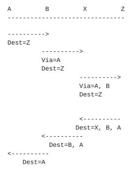
Note that the preceding Figure does not indicate whether A is a client or peer: A forwards its request to B and the response is returned to A in the same manner regardless of A's role in the overlay.
