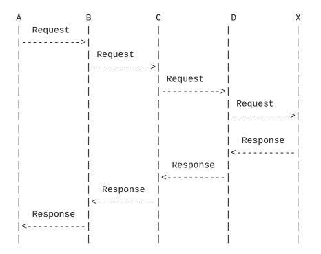
SRR works in any situation, especially when there are NATs or firewalls. A downside of this solution is that the message takes several hops to return to the peer, increasing the bandwidth usage and CPU/battery load of multiple peers.
