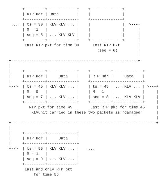
In this example, the packets with sequence numbers 7 and 8 contain portions of a KLVunit with timestamp of 45. This KLVunit is considered "damaged" due to the missing RTP packet with sequence number 6, which might have been part of this KLVunit. The KLVunit for timestamp 30 (ended in packet with sequence number 5) is unaffected by the missing packet. The KLVunit for timestamp 55,
