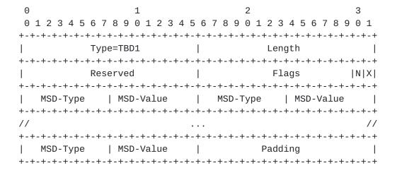
Figure 1: SRv6-PCE-CAPABILITY sub-TLV format
