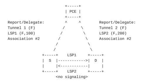
Figure 2a: Step 1: PCC-Initiated Associated Bidirectional SR Path with Forward Direction SR Paths
