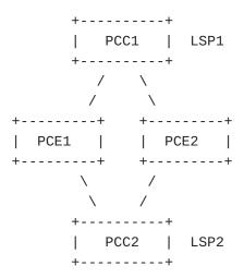
In the figure above, we consider a load-balanced PCE architecture, so PCE1 is responsible to compute paths for PCC1 and PCE2 is responsible to compute paths for PCC2. When PCE1 triggers an LSP
