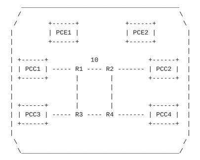
In the figure above, the requirement is to create two link-disjoint LSPs: PCC1->PCC2 and PCC3->PCC4. In the topology, all links cost metric is set to 1 except for the link 'R1-R2' which has a metric of 10. The PCEs are responsible for the path computation and PCE1 is the active primary PCE for all PCCs in the nominal case.
