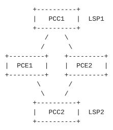
In the figure above, we consider a load-balanced PCE architecture, so PCE1 is responsible to compute paths for PCC1 and PCE2 is responsible to compute paths for PCC2. When PCE1 triggers an LSP update for LSP1, it sends a PCUpd message to PCC1 containing the new parameters for LSP1. PCC1 will take the parameters into account and will send a PCRpt message to PCE1 and PCE2 reflecting the changes. PCE2 will so be notified of the change only after receiving the PCRpt message from PCC1.
